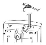
4. Route the adapter's cord through the strain relief slot on the bottom of the base.
